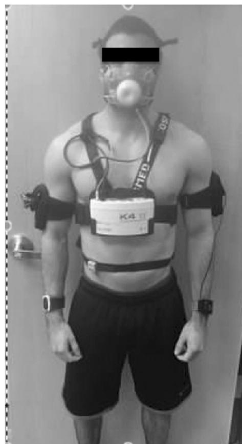
Figure 1. Participant outfitted with the K4b<sup>2</sup> (centre and face), the Mio Alpha and iPod touch<sup>®</sup> (right wrist and right arm), the Polar RS800CX (right arm); chest strap at level of xiphoid process, underneath K4b<sup>2</sup> elastic strap) and the Omron HR500U (left wrist).
